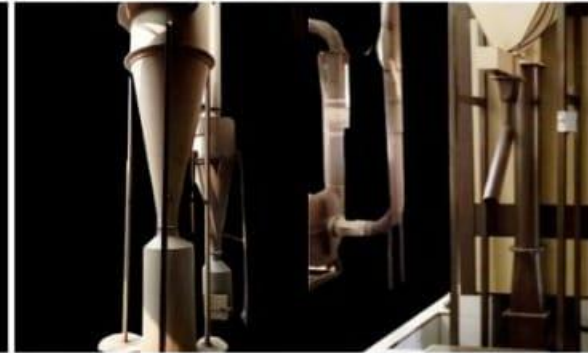
Cyclone, Roasting Fan, Destoner Collection Bean
